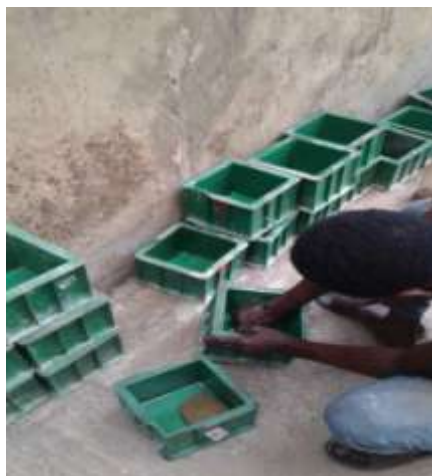
Fig. 1. Lubricating of moulds
